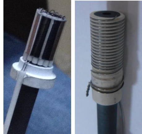
Fig. 3. a) First conventional heater design, b) Second conventional heater design
